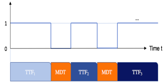
Figure 1: Sequence of Events in the Synchronous Simulation, until the TTF is reached the systems is operational and during the MDT the system is not-operational, giving a Boolean Signal of "life".
